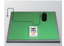
Resistance between a ground and a connecting point by a probe on a surface
