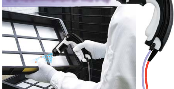
Static Elimination of the Tray
